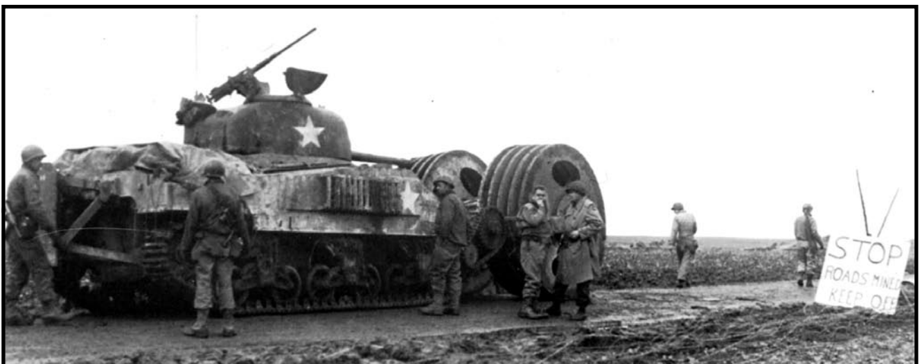
An American T1E3 'Aunt Jemima' mine-roller prepares to clean a stretch of road near Beggendorf in December 1944.
