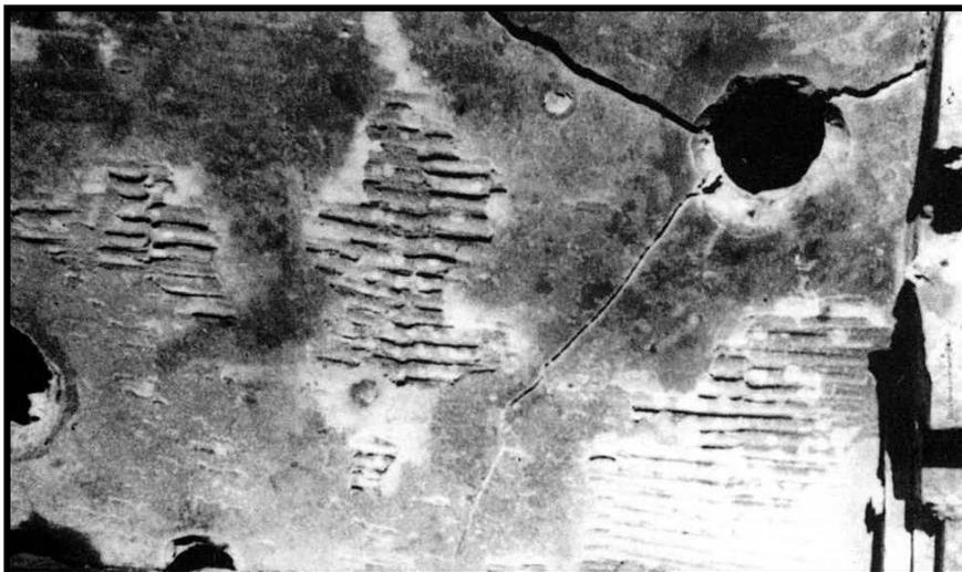
*Despite its thick armour, the Tiger II was not invulnerable. The front of this Tiger II was penetrated by a round from a IS-2, killing the driver.*
