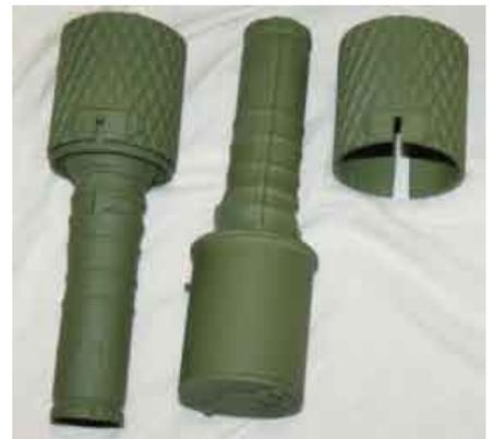
The M1933 was a replacement design for the M1914/30. Its most peculiar feature was a complex arming mechanism that required the head and handle to be turned and pulled and a safety slide operated. It worked but was overly complex. The fuse was a simple times of 4.5 to 5 seconds, activated by inertia when the grenade was thrown.
